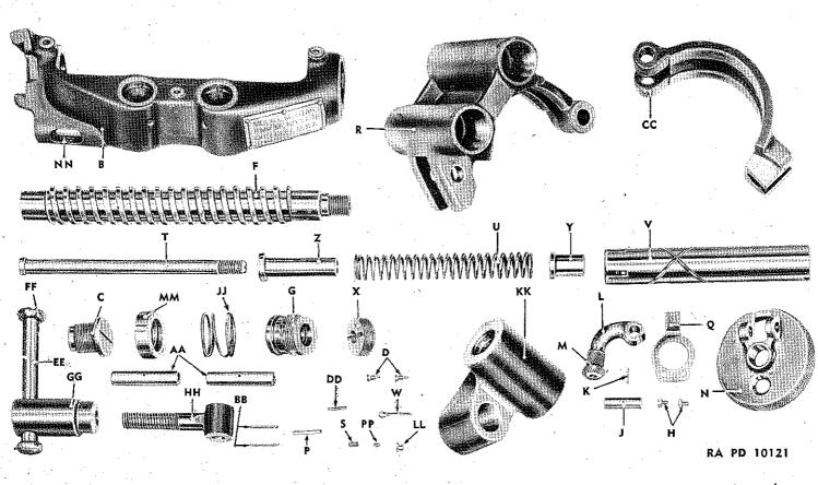
FIGURE 9 --- TRAVERSING MECHANISM GROUP PARTS FOR 81 MM MORTAR, M1 LEGEND SHOWN ON FIGURE 8
